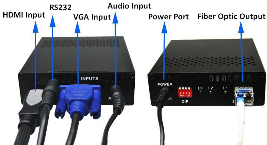
Figure 2 HD-F01-TX Fiber Optic Transmitter Connection
